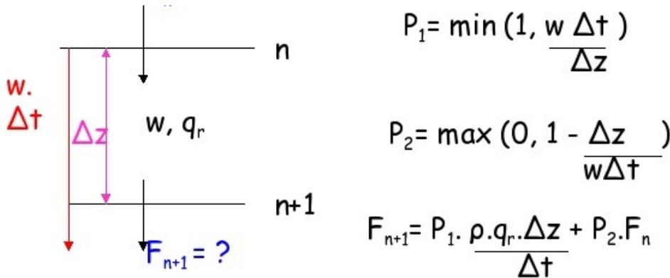
Fig. 5 : algorithm of statistical sedimentation scheme
