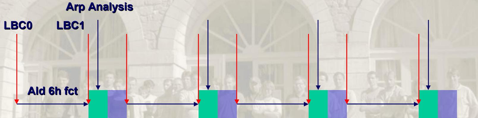
Blending: digital filter blend for 3D fields + linear combination of Surface fields, in order to combine Arpège analyzed large scales with Aladin forecast small scales
