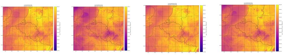
Examples of 24 hour forecasts of 2m temperature for ALARO0 run in 700m over Belgium using ALARO0 set ups with old ISBA (1&3) with SURFEX (2&4), with deep convection parametrisation on (1&2) and off (using only resolved precipitation, 3&4). Warning: the coulour range is different!
