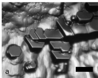
Photographs of a single crystal (a) and a bicrystal (b) after etching by sublimation with a vacuum pump in cold room. Typical facets and edges of the hexagonal system are clearly visible.
