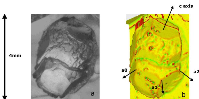
Photograph of an etch pit (a) and the replica of the same etch pit after a classical tomographic acquisition (b). The porous space was filled with 1-chloronaphthalene to preserve the figure from sublimation. Local curvature of the interface is represented to emphasize the edges and facets location (red corresponds to convex shapes of the replica, green to concaves ones).
