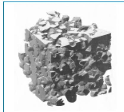
**Fig. 2(c):** melt-freeze crust, energy 10 keV.
