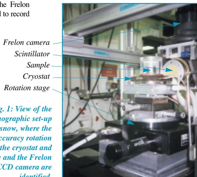
Fig. 1: View of the microtomographic set-up used for snow, where the high accuracy rotation stage, the cryostat and sample and the Frelon CCD camera are identified.
