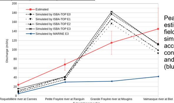
Peaks of discharge estimated by a post-flood field survey (red line), simulated by ISBA-TOP according to the different configurations (black lines) and simulated by MARINE (blue line).
