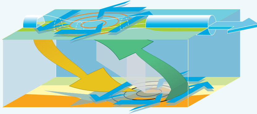
Figure SN1.6.1: Schematic representation of a developing weather system within a simple baroclinic zone. The tube is the jet-stream, blue arrows show the wind associated with the forming cyclone. The large arrows stand for the vertical motion, the ascending part of which yields precipitation.
