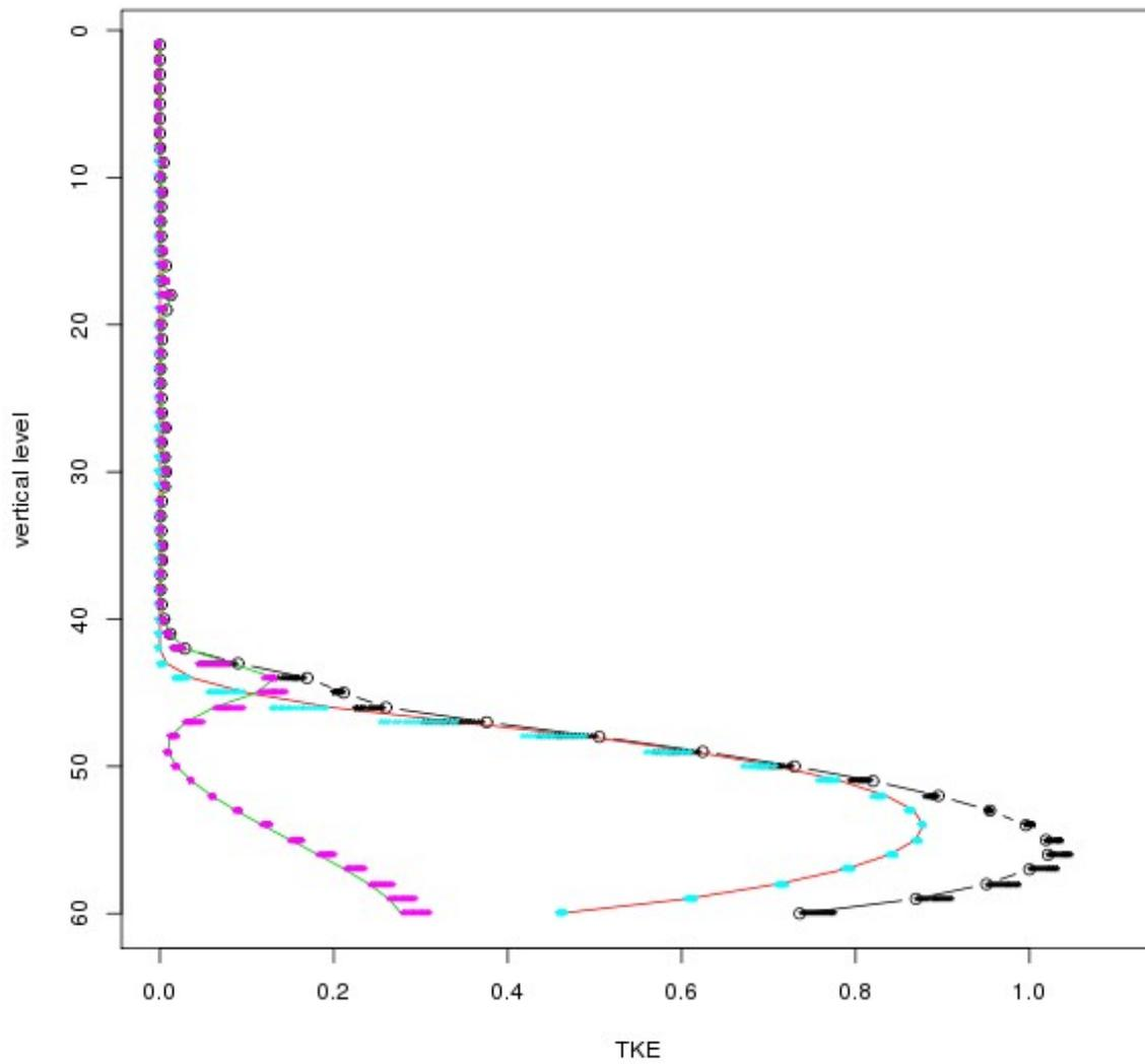
3) The vertical cross section of the average subgrid (red), resolved (green) and total (black) TKE [ $m^2/s^2$ ] at the end of the simulation. The points are the average subgrid (cyan), resolved (pink) and total (black) TKE values from the last half hour of the simulation. The grid size is 8000 m and the EDKF is turned on.
