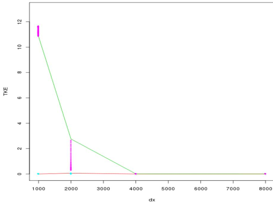
1) The average subgrid (red) and resolved (green) TKE [ $m^2/s^2$ ] on the 30. model level at the end of the simulation. The points are the average subgrid (cyan) and resolved (pink) TKE values from the last half hour of the simulation. Up - EDKF is turned on, down - EDKF is turned off.
