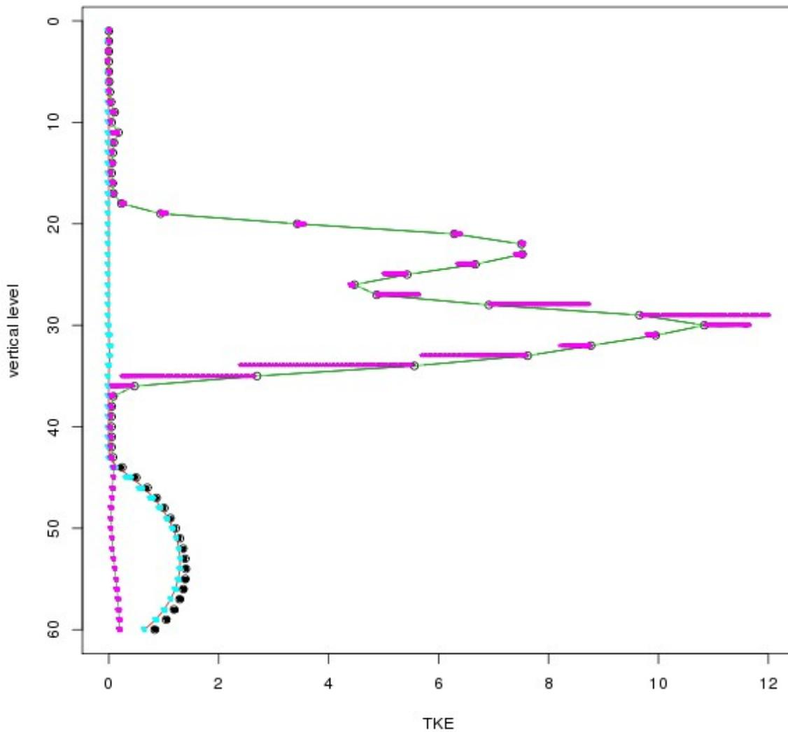
10) The vertical cross section of the average subgrid (red), resolved (green) and total (black) TKE [ $m^2/s^2$ ] at the end of the simulation. The points are the average subgrid (cyan), resolved (pink) and total (black) TKE values from the last half hour of the simulation. The grid size is 1000 m and the EDKF is turned off.
