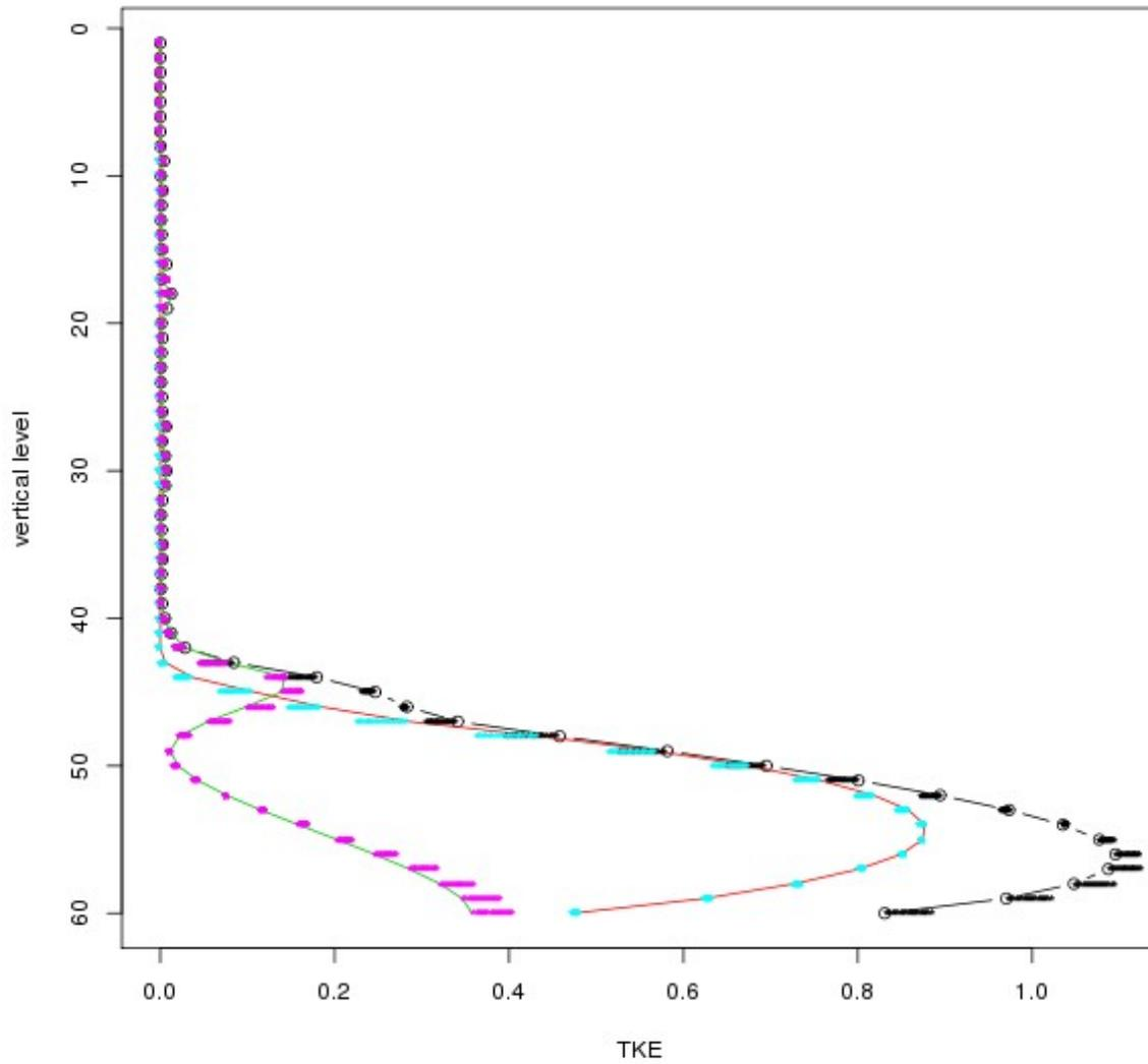
4) The vertical cross section of the average subgrid (red), resolved (green) and total (black) TKE [ $m^2/s^2$ ] at the end of the simulation. The points are the average subgrid (cyan), resolved (pink) and total (black) TKE values from the last half hour of the simulation. The grid size is 8000 m and the EDKF is turned off.
