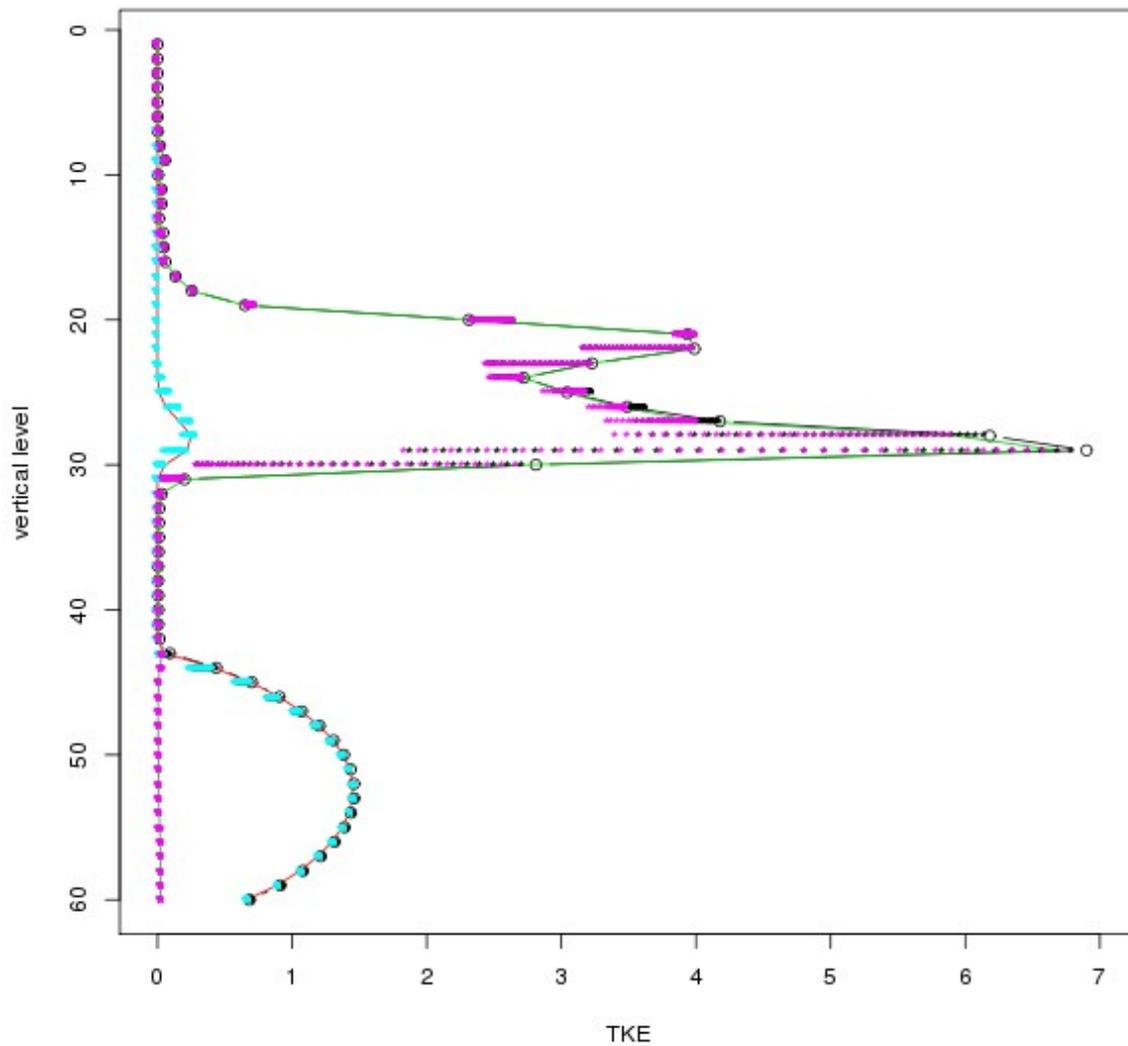
7) The vertical cross section of the average subgrid (red), resolved (green) and total (black) TKE [ $m^2/s^2$ ] at the end of the simulation. The points are the average subgrid (cyan), resolved (pink) and total (black) TKE values from the last half hour of the simulation. The grid size is 2000 m and the EDKF is turned on.
