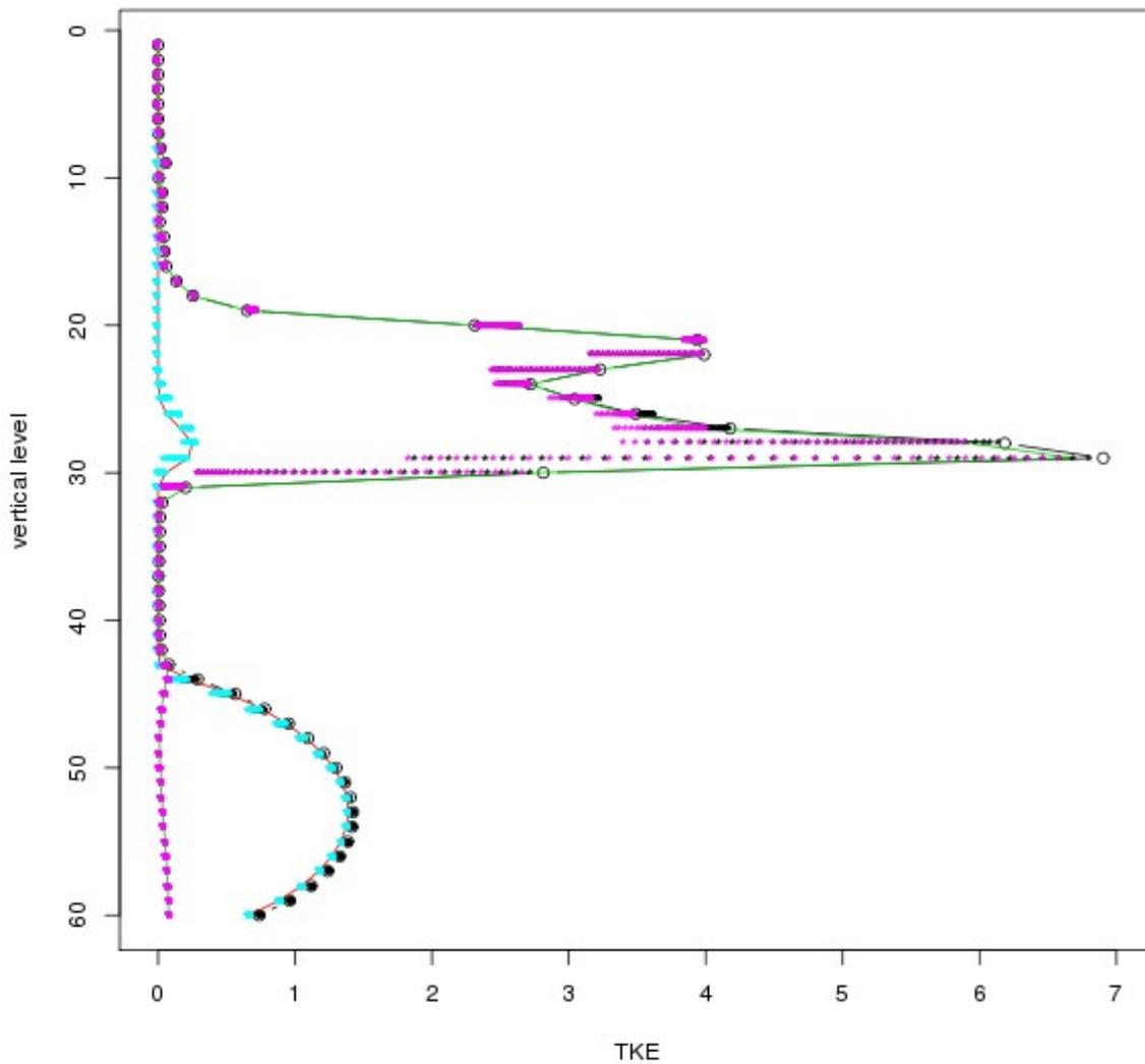
8) The vertical cross section of the average subgrid (red), resolved (green) and total (black) TKE [ $m^2/s^2$ ] at the end of the simulation. The points are the average subgrid (cyan), resolved (pink) and total (black) TKE values from the last half hour of the simulation. The grid size is 2000 m and the EDKF is turned off.
