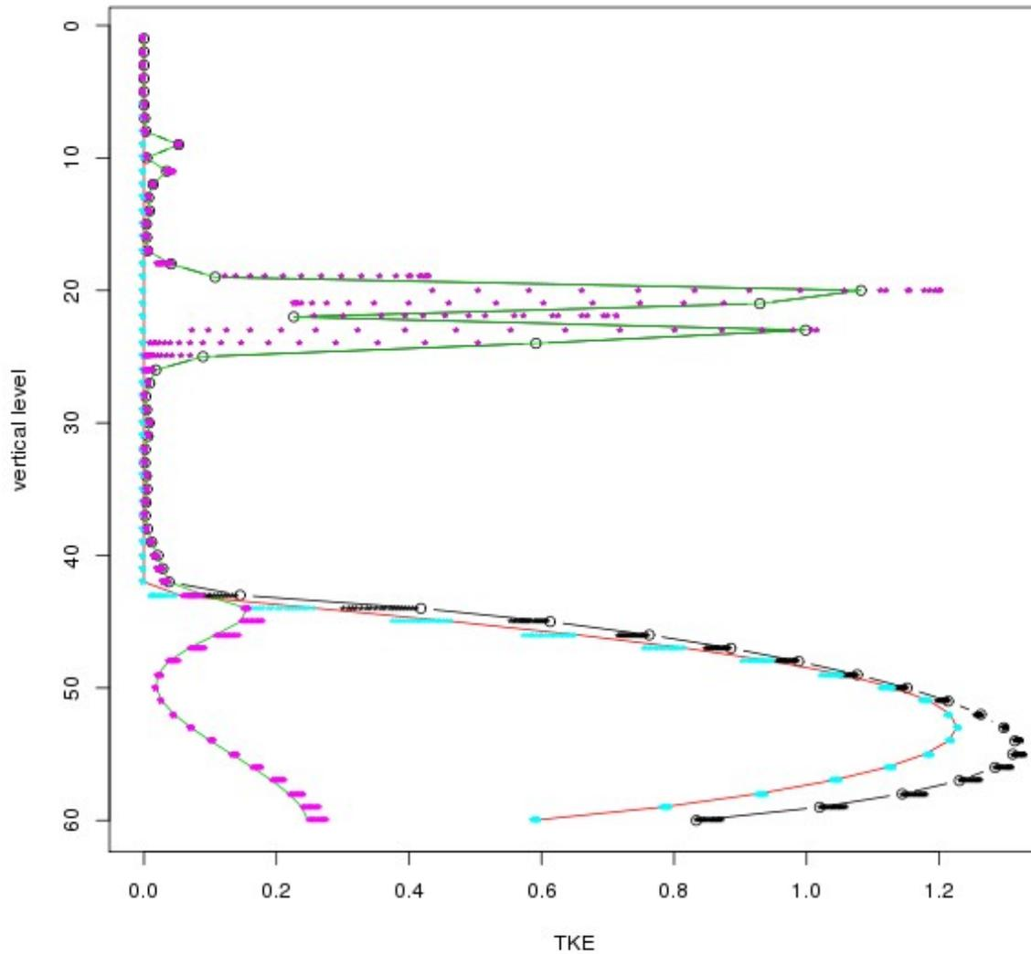
6) The vertical cross section of the average subgrid (red), resolved (green) and total (black) TKE [ $m^2/s^2$ ] at the end of the simulation. The points are the average subgrid (cyan), resolved (pink) and total (black) TKE values from the last half hour of the simulation. The grid size is 4000 m and the EDKF is turned off.
