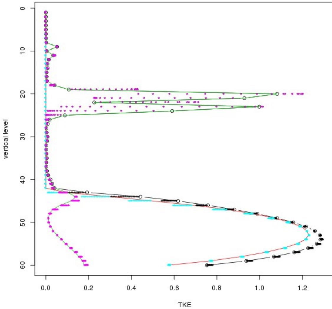
5) The vertical cross section of the average subgrid (red), resolved (green) and total (black) TKE [ $m^2/s^2$ ] at the end of the simulation. The points are the average subgrid (cyan), resolved (pink) and total (black) TKE values from the last half hour of the simulation. The grid size is 4000 m and the EDKF is turned on.
