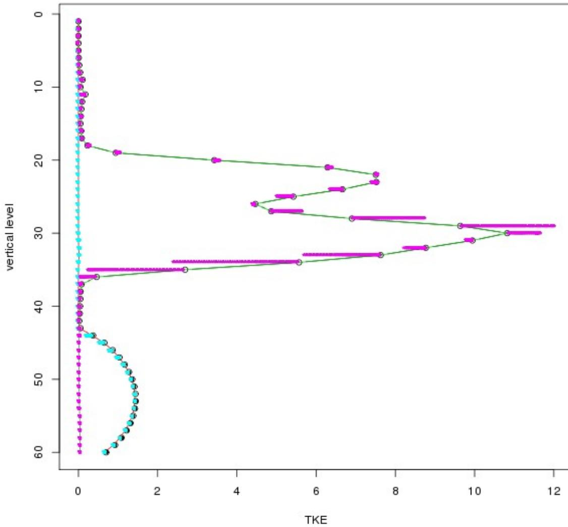
9) The vertical cross section of the average subgrid (red), resolved (green) and total (black) TKE [ $m^2/s^2$ ] at the end of the simulation. The points are the average subgrid (cyan), resolved (pink) and total (black) TKE values from the last half hour of the simulation. The grid size is 1000 m and the EDKF is turned on.
