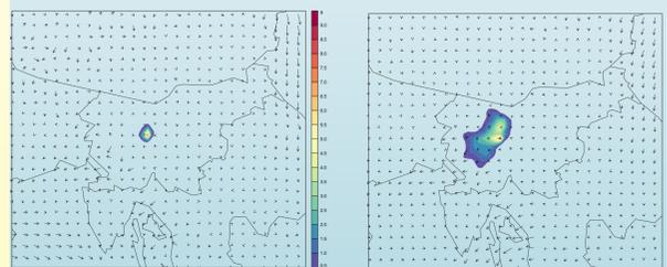
First tests with single source, concentration of SO<sub>2</sub> [µg/m<sup>3</sup>] after 5 and 10 hours of simulation.
