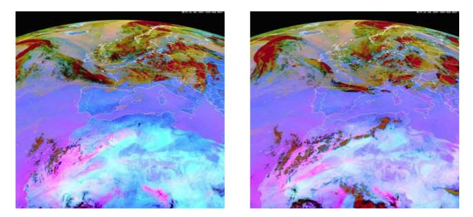
Fig.4 The RGB composite dust product of EUMETSAT for July 10th at 12H00 and 18H00 (dust is represented by the magenta colour)
