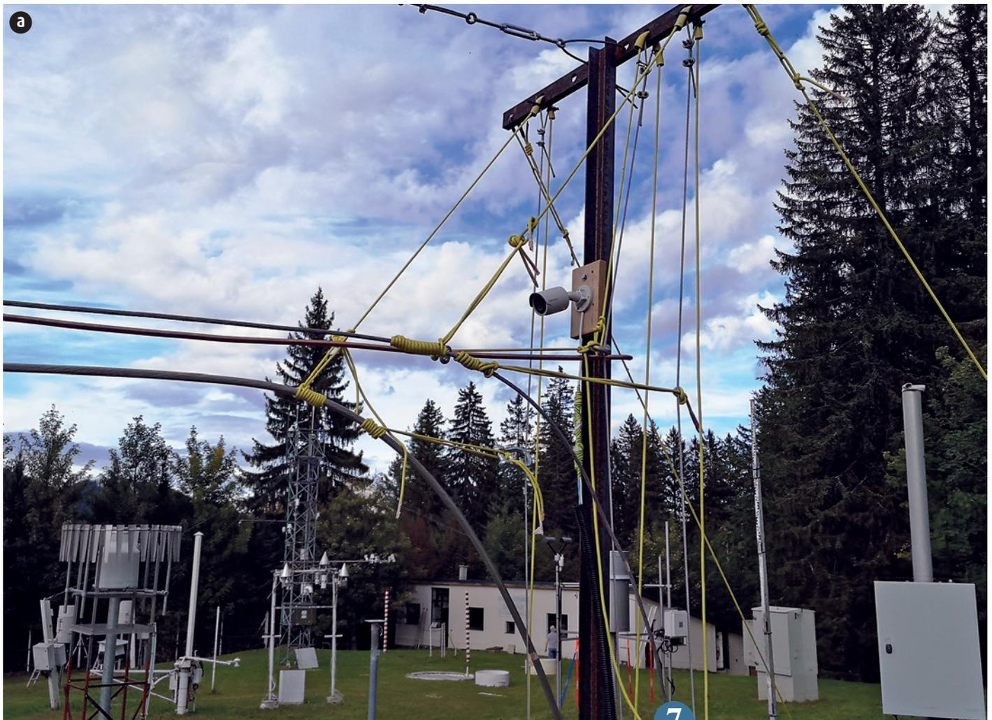
(a) Experimental site dedicated to observation of snow and ice accretion events on transmission overhead wires (RTE and ENEDIS electricity transportation wires, SNCF catenary) located at Col de Porte.
