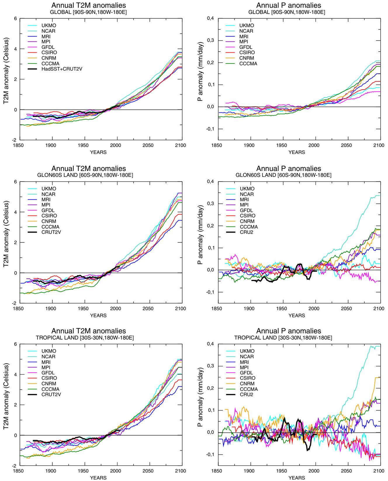
**Fig. 2** Transient 11-year moving average response of annual mean surface air temperature (*left panels*) and annual mean precipitation (*right panels*) to anthropogenic radiative forcing relative to the 1971–2000 model climatologies. The results are shown for global
