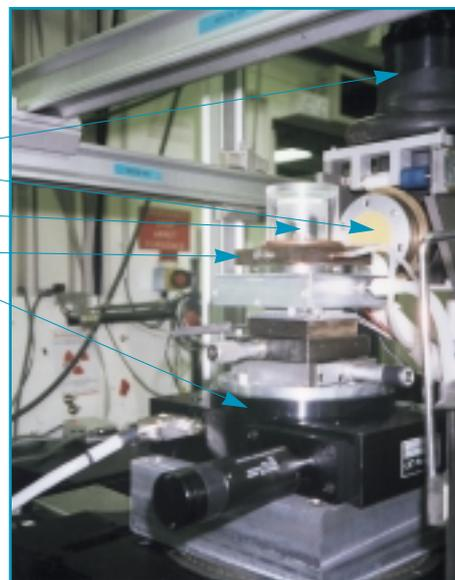
*Fig. 1: View of the microtomographic set-up used for snow, where the high accuracy rotation stage, the cryostat and sample and the Frelon CCD camera are identified.*
